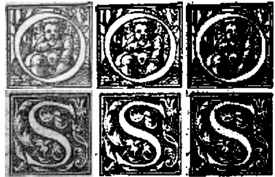
Figure 5. Examples of Otsu's adaptive thresholding for ornamental letters. From left to right: original image, Otsu optimal thresholding ( \alpha = 0 ) and our method ( \alpha = 0.5 ).
